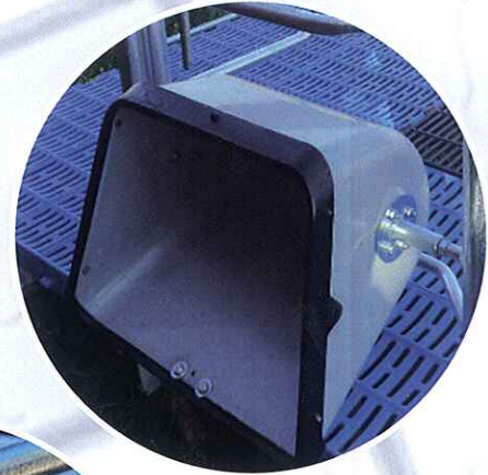
Hranilica se može oboriti radi pranja Feeders for sows can go down for cleaning
